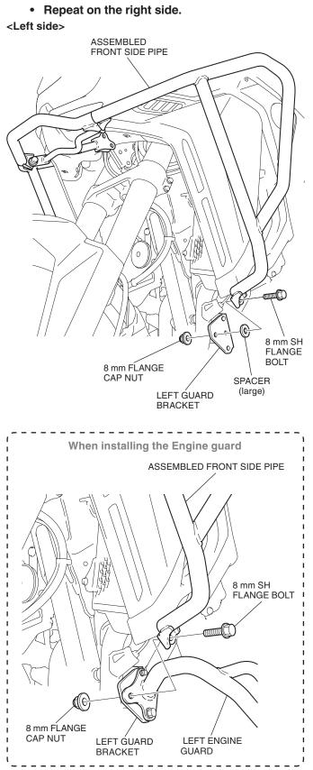
25. Raise and install the assembled front side pipe as shown.
