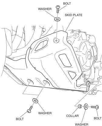
Remove the skid plate as shown.
