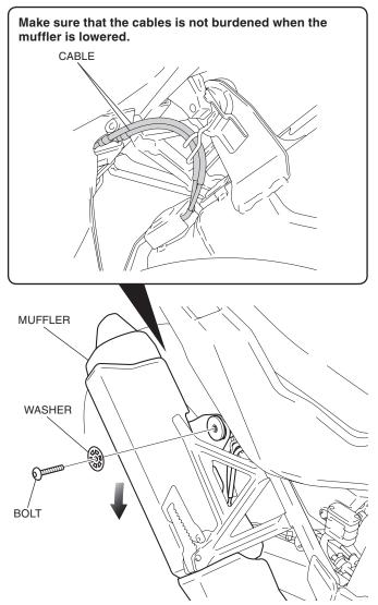
12. Remove the parts as shown. **<Left side>**
