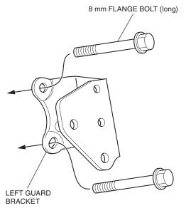
14. Install the left guard bracket as shown. **<Left side>**
