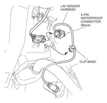
5. Remove the bosses of the right middle cowl, drain tube and LAF sensor harness in the same manner as the left side.
